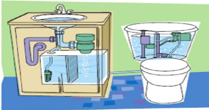
Figure 33 : Plumbing fixtures that use gray water from sinks for flushing toilets
